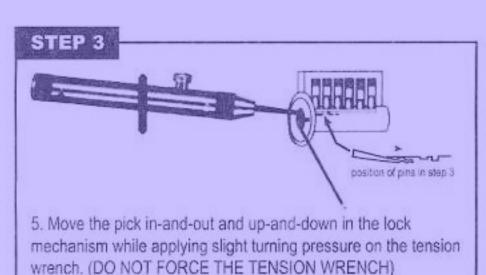
The pick begins to line up the pins to a shear line as the tension wrench applies slight pressure to prevent the pins from dropping back down.
